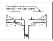
Secure the drain flange to the roof deck/ nailer using a minimum of three pan-head fasteners, evenly spaced around the flange. The flashing membrane must cover and extend past the fas-tener head. Flashing membrane must be installed per roof membrane manufacturer's detail.
