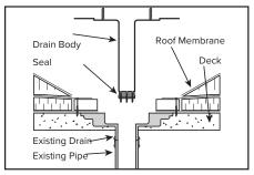
Examine the existing water leader to make sure there are no elbows that prevent the drain stem from being fully inserted into the pipe. Insert seal into end of drain stem and tighten screws enough to hold the seal in place during installation. Insert assembled drain into existing leader pipe until flange lies flush on roof membrane.
